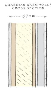
Cross section based on Kingspan TEK building system, including exterior finish, battens and plasterboard.
