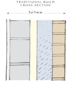
Cross section based on exterior brick, cavity, PIR insulation, blocks and plasterboard.
